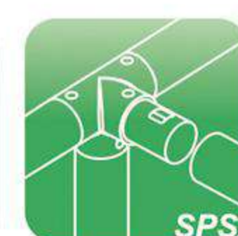
H Angle Plate For the connection between side base and frame profile at the 90^\circ corner of the platform.
